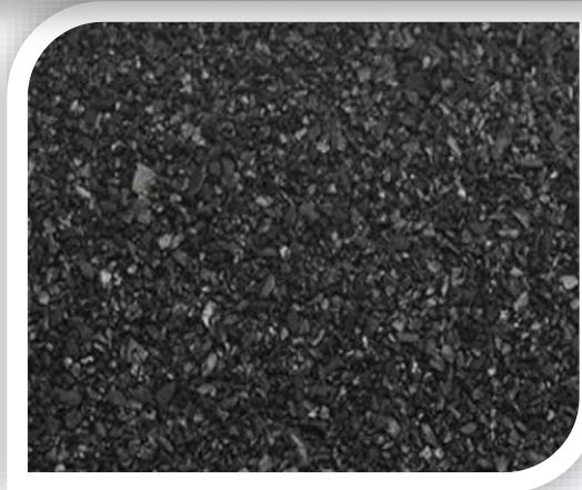
High-quality activated carbon is used in air and gas plants for the removal of oil vapors, hydrocarbons, odors, and organic impurities. Its highly porous structure provides a large surface area for efficient adsorption, protecting downstream equipment and improving gas purity. It plays a critical role in air purification and pre-treatment stages of PSA and gas generation systems.
