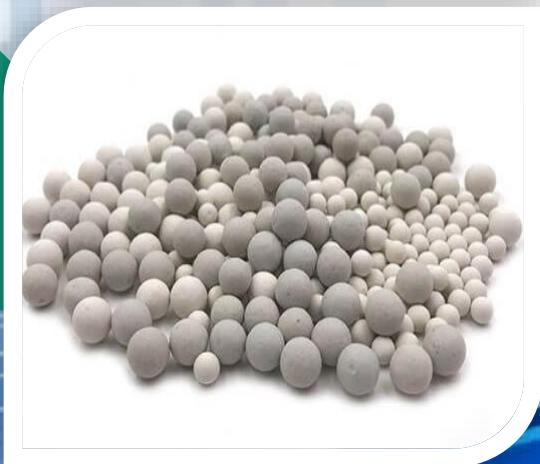
Ceramic balls are used as inert support media in gas plants and process vessels to ensure uniform gas flow and proper distribution of adsorbents or catalysts. They provide mechanical support, prevent channeling, and enhance system efficiency. Due to their high compressive strength, thermal resistance, and chemical inertness, ceramic balls ensure reliable and long-term operation.
