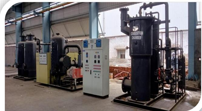
**GAS PURITY: CO: 18% – 22%, H<sub>2</sub>: 2% – 5%, CO<sub>2</sub>: 4% – 8% & N<sub>2</sub>: Balance**
