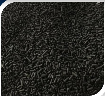
Carbon Molecular Sieve is a specialized adsorbent used in PSA nitrogen gas generation systems based on selective adsorption of oxygen molecules. Its controlled pore structure allows rapid oxygen separation while retaining nitrogen, ensuring stable purity levels, consistent performance, and long service life under continuous industrial operation.
