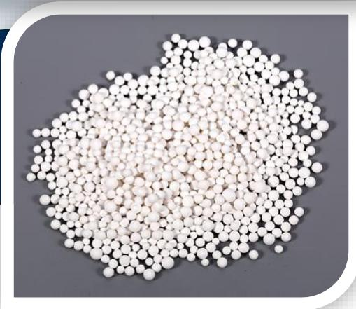
Activated alumina is a highly porous aluminum oxide adsorbent used for deep drying and moisture removal in compressed air and gas systems. It works on the principle of physical adsorption, ensuring low dew point levels and stable system performance. Its high mechanical strength, thermal stability, and long service life make it ideal for desiccant air dryers and gas purification applications.
