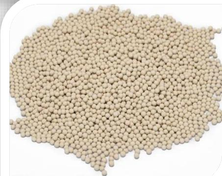
Zeolite Molecular Sieve is a crystalline aluminosilicate adsorbent used in PSA and VPSA oxygen generation systems. It selectively adsorbs nitrogen under pressure, enabling the production of high-purity oxygen with reliable cycle performance, high adsorption efficiency, and proven durability in medical and industrial applications.
